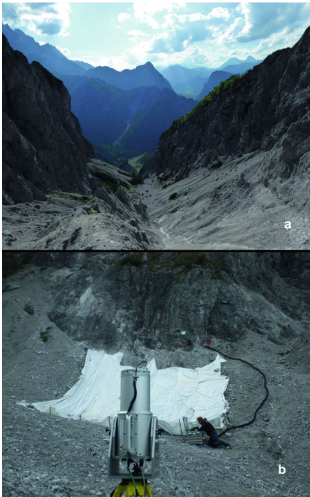
Fig. 18.9 Gsenggraben. a Overview of the catchment area, as seen from the head of the valley, looking towards west. b View of one of the investigated rockwalls showing the terrestrial laser scanner, the rockfall net and the cables of the sensor instrumentation. Photos: A: G.K. Lieb, B: M. Rode
