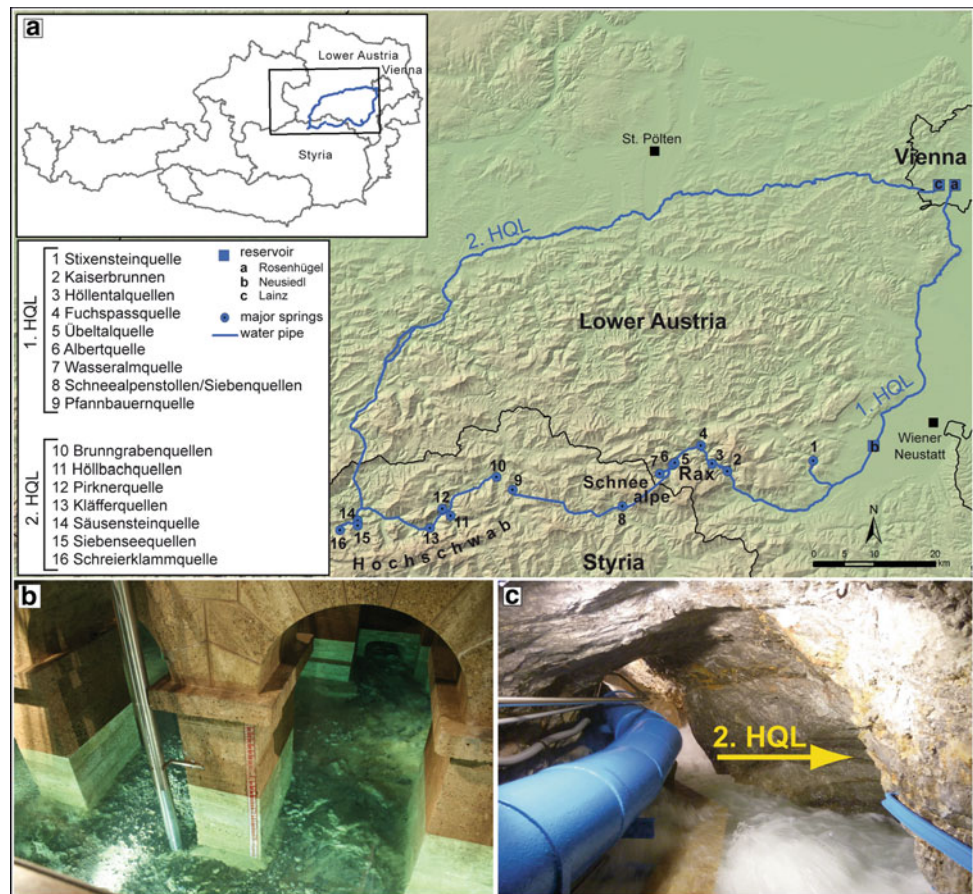
Fig. 5.13 Vienna water supply. a Map and main developed springs (HQL = Hochquellenleitung). b Spring tapping of the Kaiserbrunnen. c Spring tapping of the Kläfferquellen; Photographs: C. Bauer
